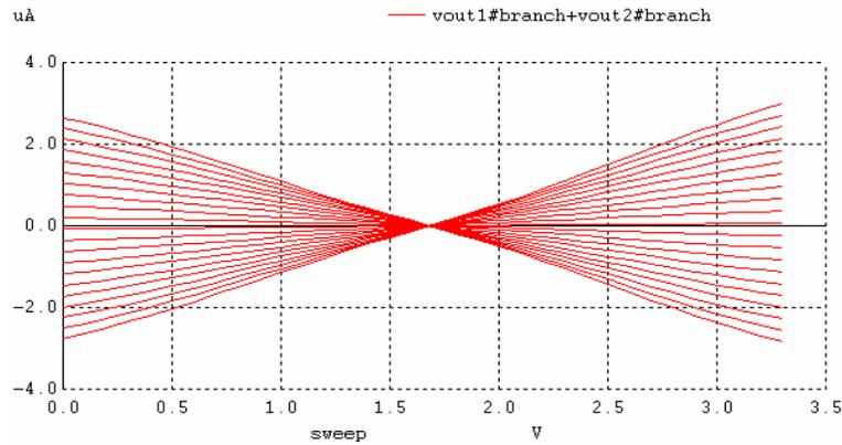
**Figure 2.  $I_{out}$  versus  $V_w$  and with  $V_{in}$  as a parameter.**
