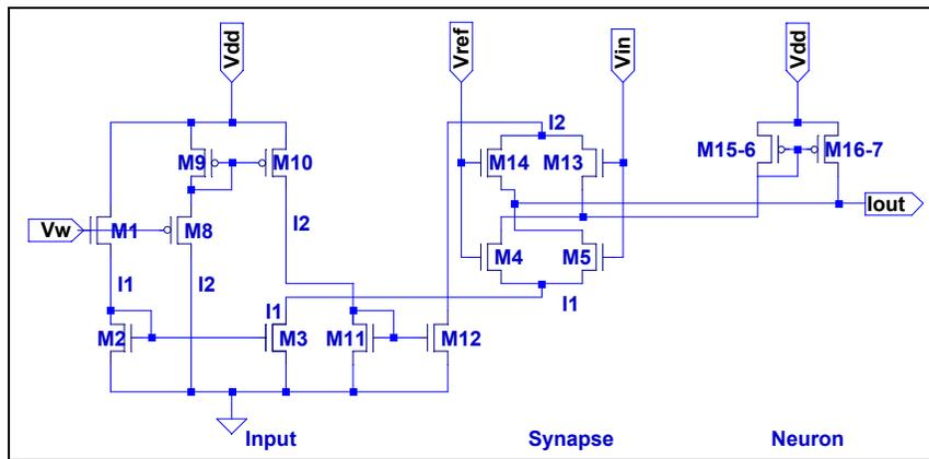
Figure 1. The multiplier circuit.
