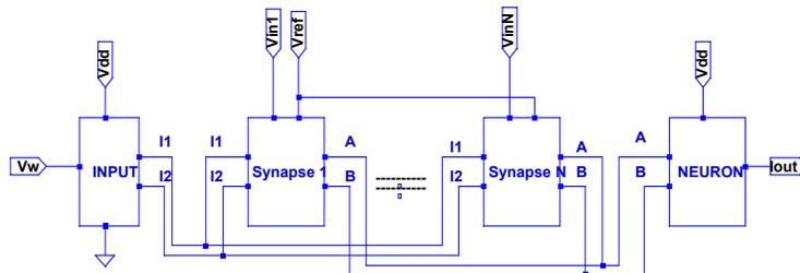
Figure 9. N synapses connected to one neuron.
