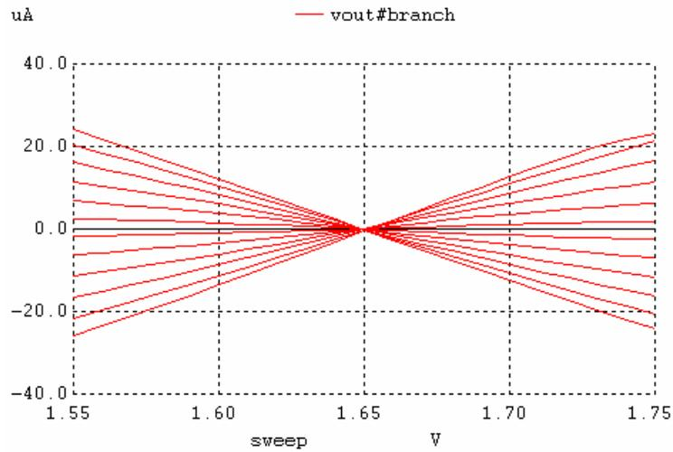
Figure 11.  $I_{out}$  versus  $V_w$  and with  $V_{in}$  as a parameter (ten synapses connected to one neuron).
