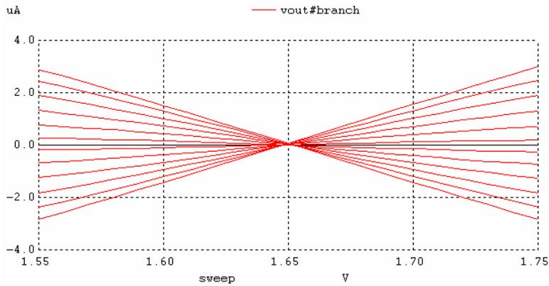
**Figure 3.  $I_{out}$  versus  $V_{in}$  and with  $V_w$  as a parameter.**
