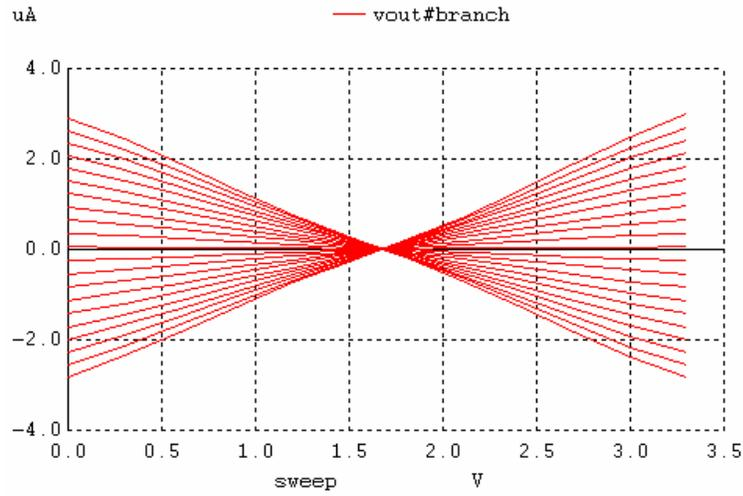
Figure 10.  $I_{out}$  versus  $V_w$  and with  $V_{in}$  as a parameter (one synapse connected to one neuron).
