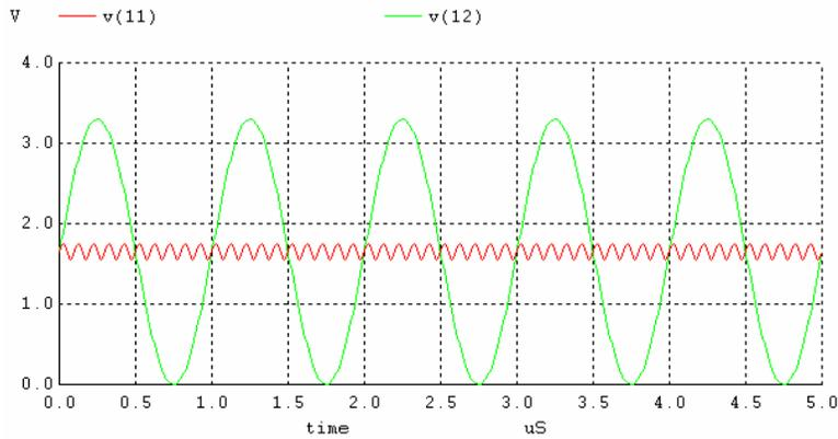
Figure 4. The multiplier two input sinusoidal voltages  $V_{in}$  and  $V_w$ .
