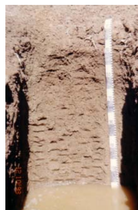
Figure 2. Sampling was done from the water table up to the soil surface to avoid cross contamination of soil samples.
