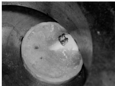
Figure 1. Tooth specimen during shear testing. Load applied perpendicular to the bracket/enamel interface.
