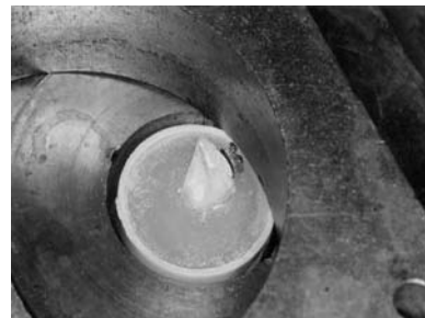
Figure 2. Tooth specimen during tensile testing. Load applied perpendicular to the bracket/enamel interface.
