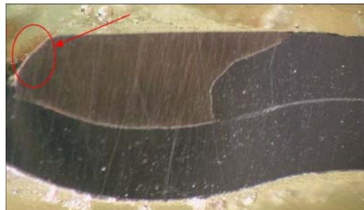
Figure 9. Detail of corrosion attack in right-hand brazing, extension of 10x.
