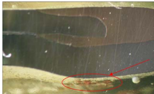
Figure 8. Detail of corrosion attack in left-hand brazing, extension of 10x.
