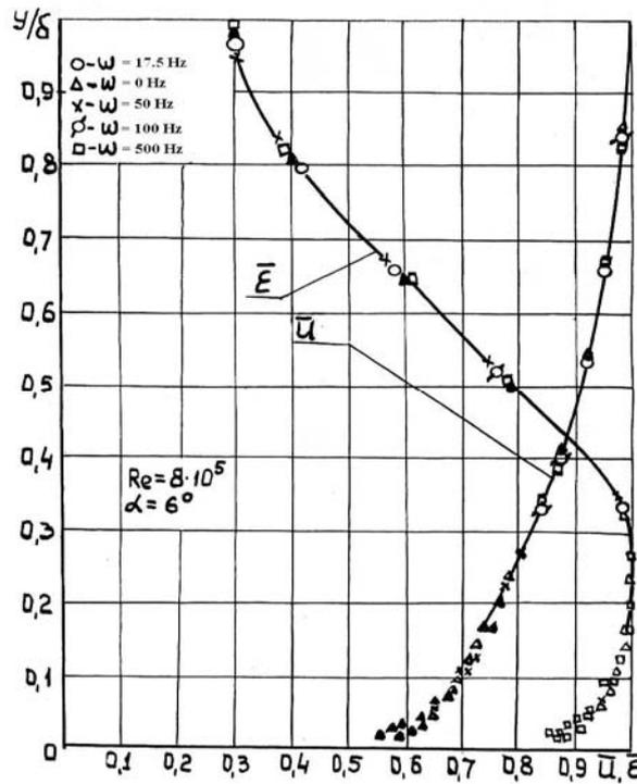
**Figure 5. The distribution of the velocity profiles and the relative turbulence number across the boundary layer on a vibrated wall.**
