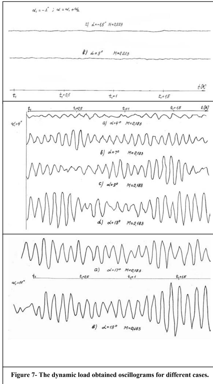
Figure 7- The dynamic load obtained oscillograms for different cases.
