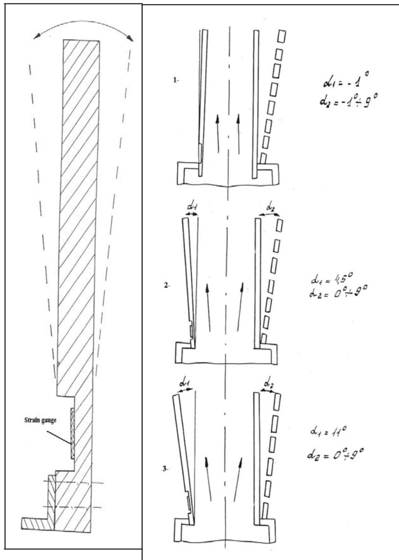
Figure 6. The plane passage in different plate's positions, and the upper plate with a strain gauge to record the dynamic loads.
