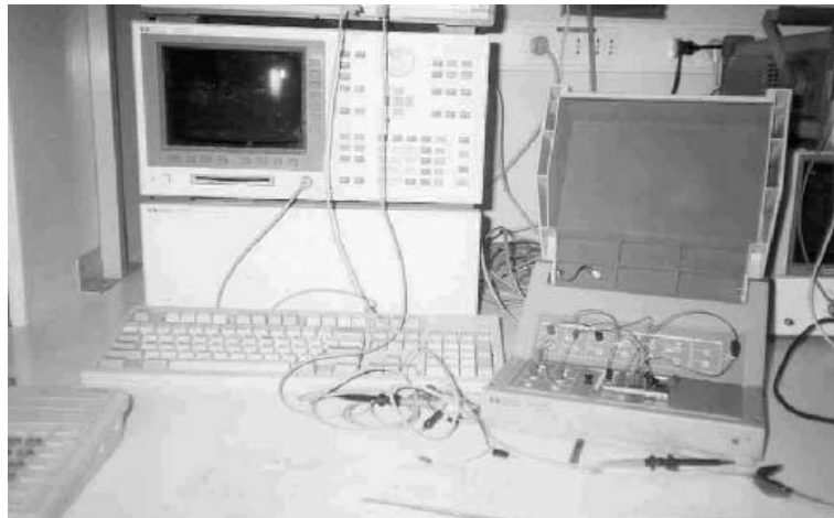
Figure 5. The logic state analyser system to test and measure the circuit.
